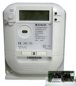
Figure 6.8: Echelon Smart Meter with MEP card, for measuring electricity consumption, collect and send data from other smart meters/devices (e.g., from the smart meters for water and district heating)
