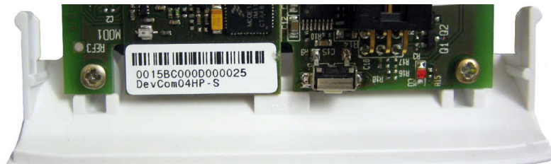
Figure 4.1: DEVELCO MEP card for electricity meters
