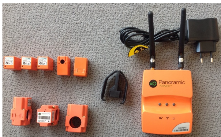
Figure 4.2: Panoramic Power sensors
